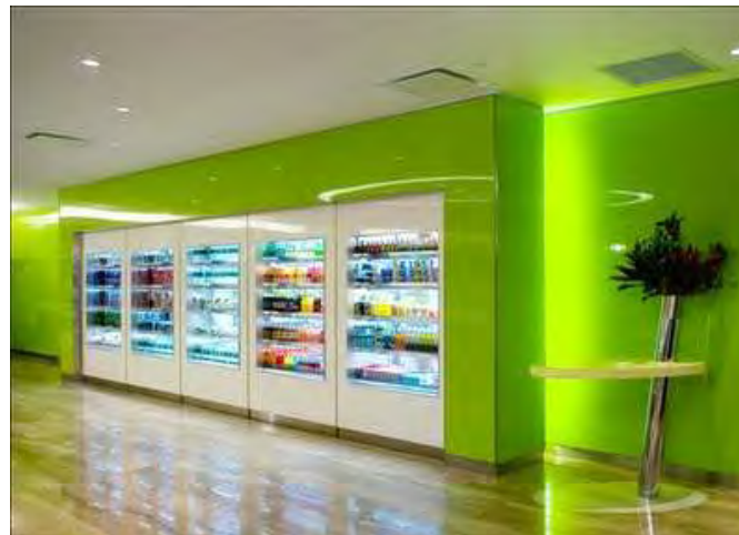
Figure 49: Example of color and cove wall lighting
