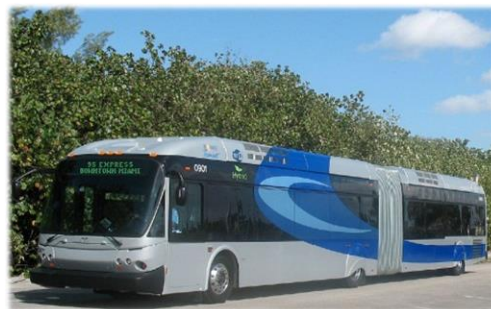
FIGURE 1: ARTICULATED DIESEL HYBRID-ELECTRIC BUS USED FOR THE I-95 EXPRESS SERVICE TO MIAMI BY BROWARD COUNTY TRANSIT.
