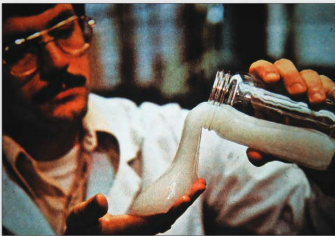
Figure 7. Example of a gel used in hydrofracturing to carry proppant into a fracture. Photograph by Daniel Soeder, USGS.
