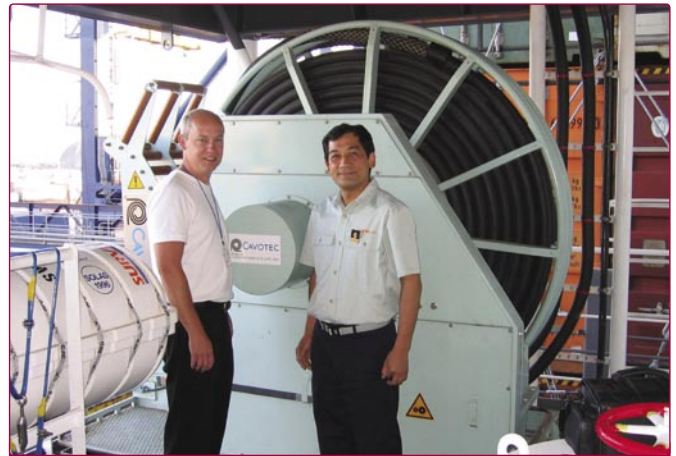
Figure 1. Electrical cable reel on ship.
