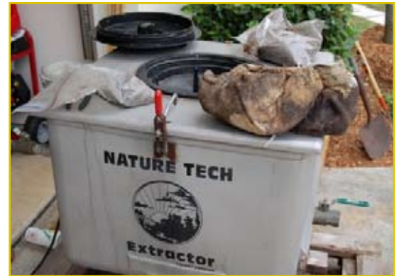
40 gallon extrator with compost used to produce highly concentrated living microbes.
