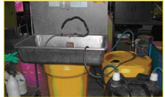
Recycling water-based parts washer. The recycling action extends the life of the cleaner, thus the facility uses less.
