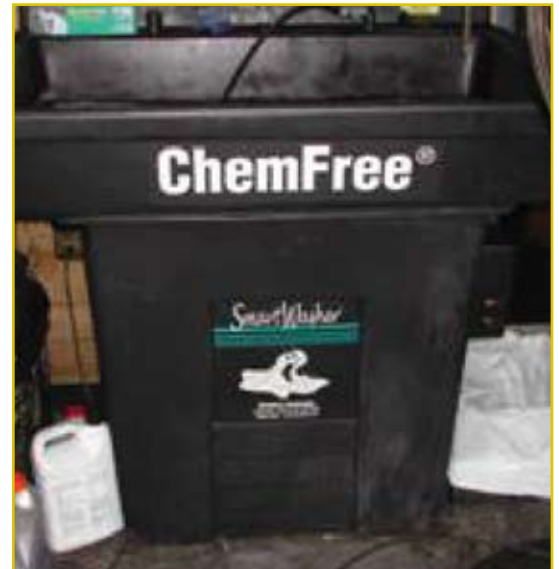
Replaced toxic mineral spirits to clean parts by installing ChemFree -- a water- and enzyme-based parts washer.
