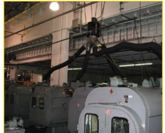
The mist-collection system removes oil particles from air and recycle to machines.
