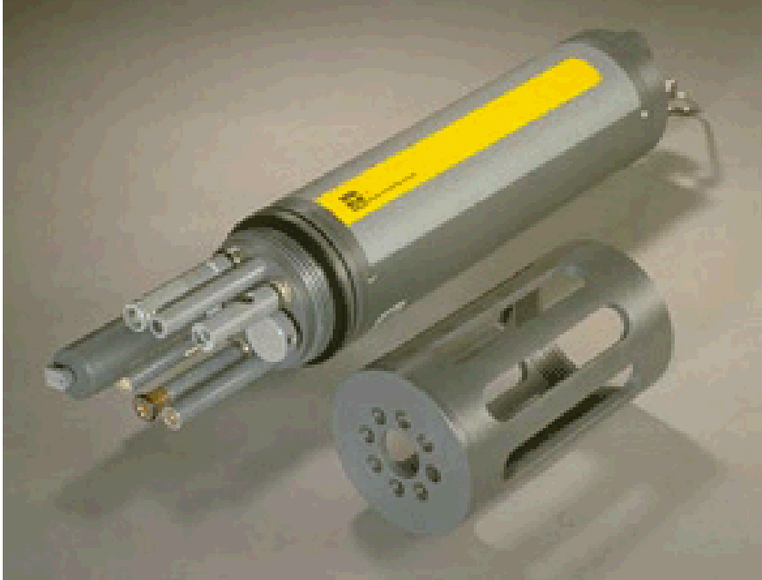
Figure 6a. YSI Data Sondes Similar to the Ones Deployed at Snake Warrior’s Island Natural Area. The sondes measure temperature, pH, water elevation, dissolved oxygen, chlorophyll and turbidity. The sondes were programmed to log readings every 15 minutes. Sondes were deployed inside PVC housings for a week at a time in wetland 3 and the retention pond at Snake Warrior’s Island Natural Area.
