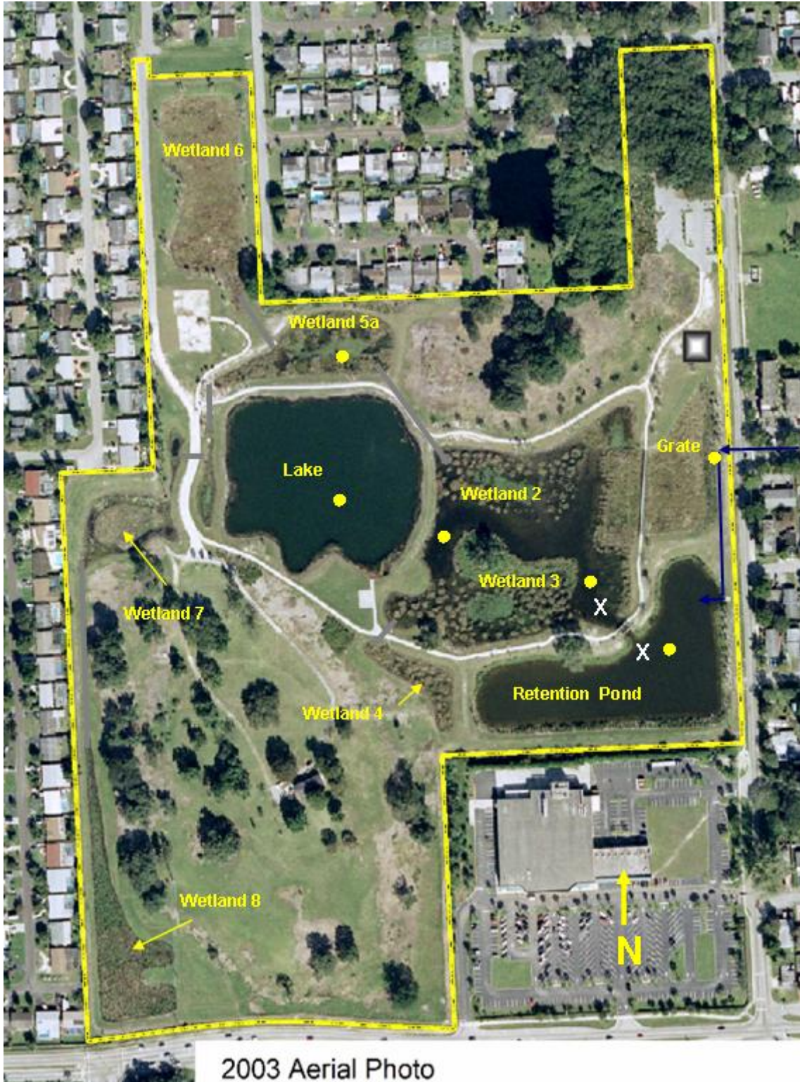
Figure 5. 2003 Aerial Photograph of Snake Warrior's Island Natural Area. X's indicate the location of the two YSI data sondes. Bullets (●)'s indicate the locations of the monthly sample sites at Snake Warrior's Island Natural Area. The blue arrows show where surface water and storm water enter SWI.
