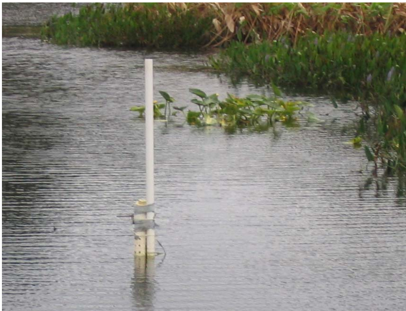
Figure 6b. PVC Housing Containing One of the Sondes Deployed at Snake Warrior’s Island Natural Area. This sonde is located in wetland 3.
