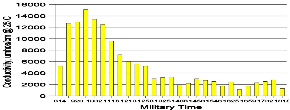
**Figure 14: Sewage Conductivity Readings, Isle of Venice Pump Station, March 2, 1995**
