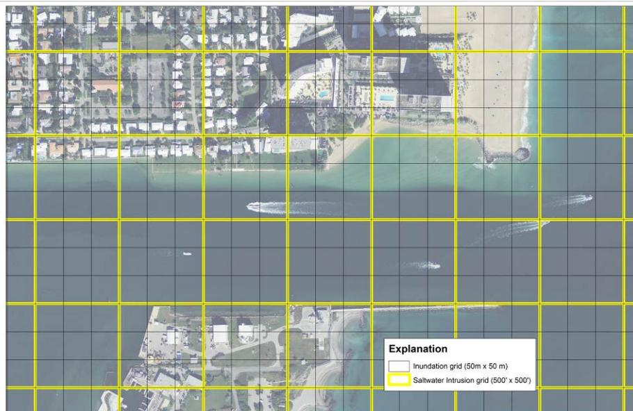
Figure 2. Grid discretization used in Inundation focal areas (50x50m =165x165ft) vs. the larger grid used in the Variable Density Models (500x500ft).
