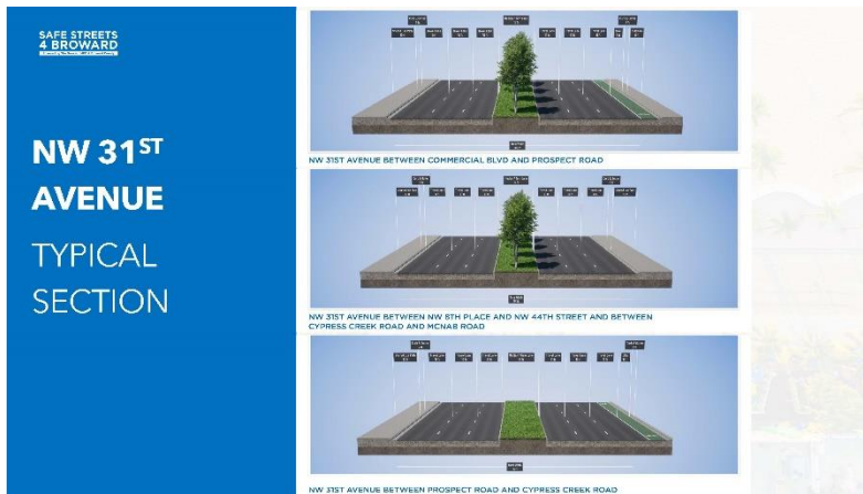
Figure 23: Slide 24 NW 31st Avenue Typical Section
