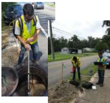
Figure 6: Example force main field assessment at JEA using BEM
