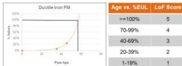
Figure 7: Example ductile iron force main deterioration curve developed with Lee County, FL
