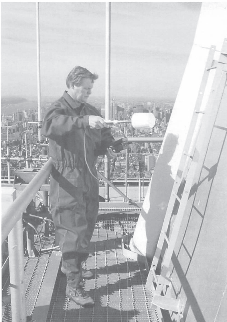
Figure D-4. Photograph of RF protective suit being used during an RF survey.
