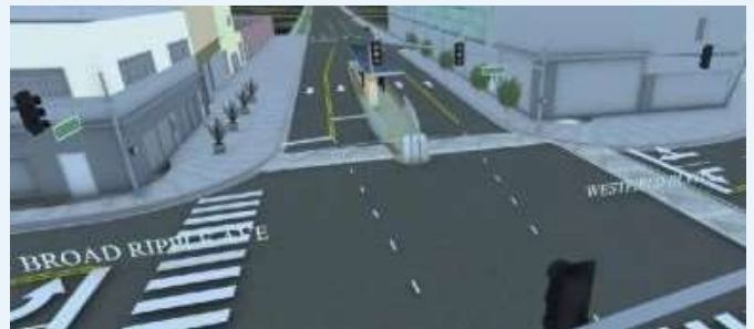
CDM Smith has developed an innovative approach to improvement development and visualization which provides dynamic visualization through 3D flyover video and fully immersed virtual experience. Improvements are developed in 3D, based on horizontal, vertical, and cross-sectional elements, to show a detailed 3D view of the design such as the image above, showing the IndyGo Red Line BRT station at College and Broad Ripple. The model can be efficiently converted to a 3D flyover video to further emphasize the visual message and clearly communicate to the public how the station will look and function at specific locations.
