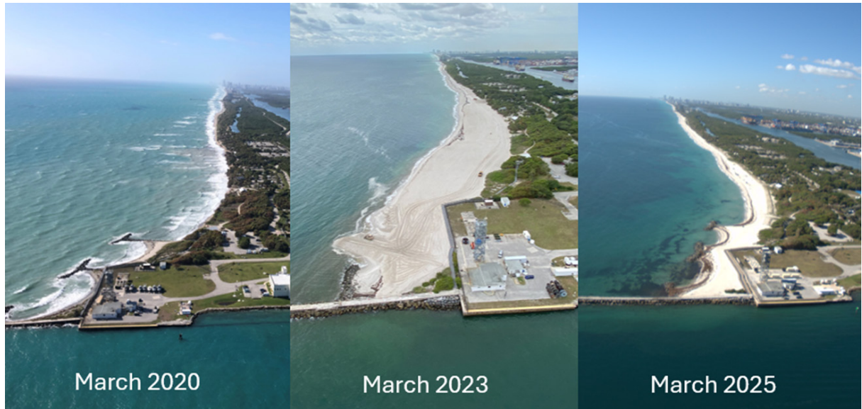
Photo showing the shoreline south of the Port Everglades Inlet over time – before traditional beach nourishment (March 2020), immediately after sand placement (March 2023), and just two years later (March 2025). This area experiences the highest rate of erosion in Broward County, demonstrating the critical need for the Sand Bypass Project.
