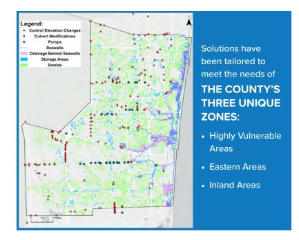
**Tier 2 (By 2070):** Addresses the challenges of a projected 3.3-foot rise in sea levels by 2070. In addition to the adaptations under Tier 1, this phase involves raising seawalls to 7.0 feet NAVD for enhanced coastal protection and adding advanced drainage systems, including pumping and collection systems to manage increased stormwater volumes behind seawalls. Tier 2 also expands green spaces further to mitigate urban heat and enhance biodiversity.
