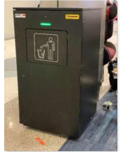
Figure 87: Automatic Compacting Trash Receptacles at FLL Terminal 2
