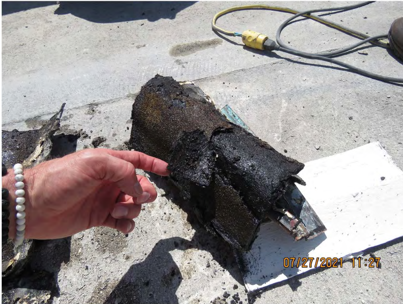
This is the sample taken from the above photograph showing the rotted wood fiber coverboard and moisture in the roof system.
