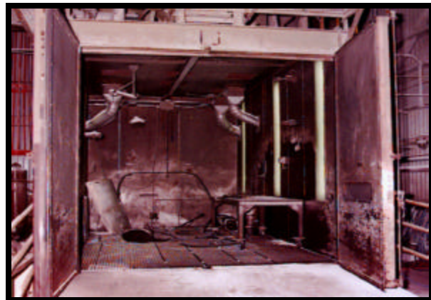
An abrasive blasting booth for cleaning parts. Photo Courtesy of NADEP Jacksonville
