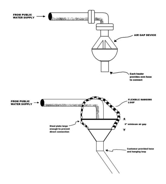
FIGURE 1 – SUGGESTED FILLING DEVICE FOR WATER LOADING STATIONS
